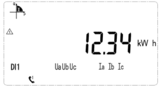
Current reversing active energy 12.34kWh
