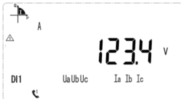
Voltage on A phase is 123.4V
