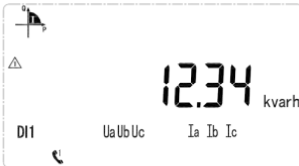
Current forward reactive energy 12.34kWh
