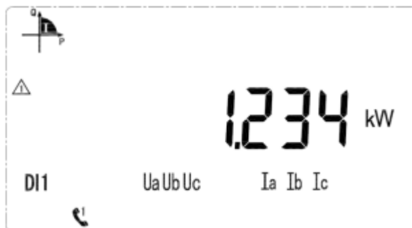
Current total power is 1.234kW
