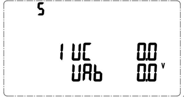
Phase voltage U_c and line voltage U_{ab}
