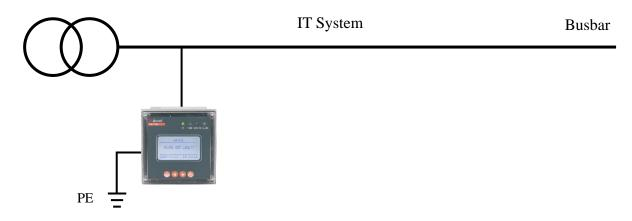
**Instructions:** Stand-alone IT systems typically use a single insulation monitor, and the simultaneous operation of multiple insulation monitors can cause signal interference problems.
