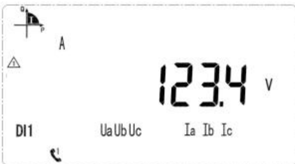
Voltage on A phase is 123.4V
