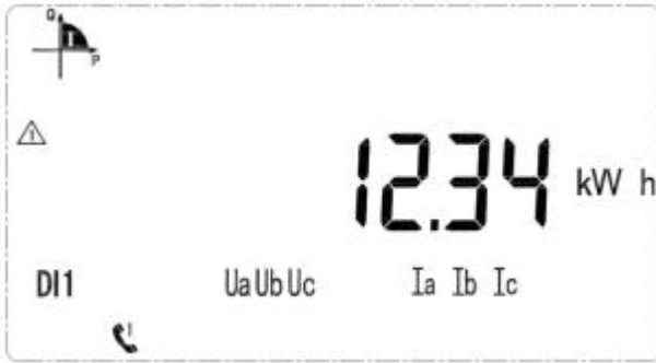
Current forward active energy 12.34kWh
