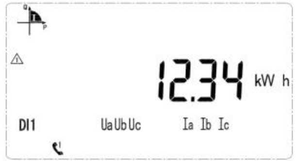
Current reversing active energy 12.34kWh
