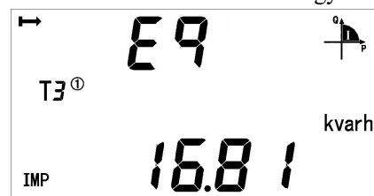
Current forward reactive total energy
