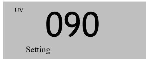
Figure 99 Undervoltage Protection Settings
