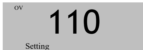
Fig. 31 Overvoltage protection Settings
