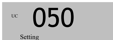
Fig. 34 Undercurrent protection Settings
