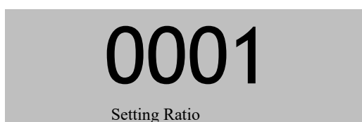
Fig. 93 Current transformer ratio setting
