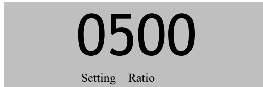
Fig. 26 Current transformer ratio setting
