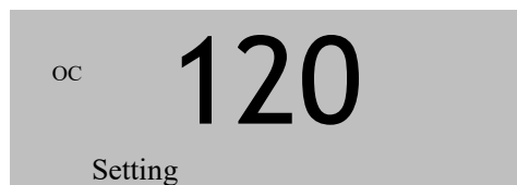
Fig. 33 Overcurrent Protection Settings
