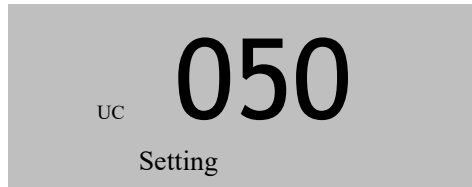
Fig. 48 Undercurrent protection Settings
