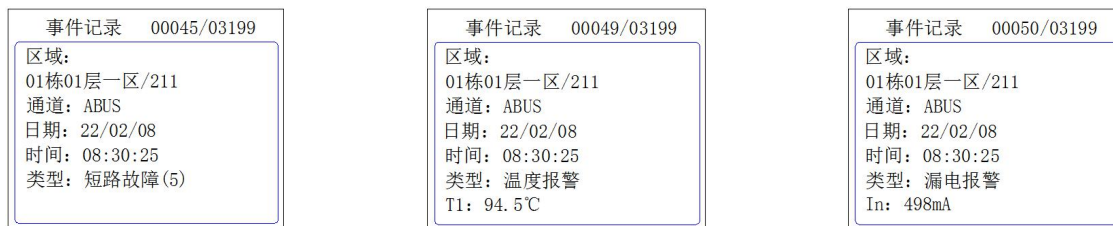
短路故障 Short-circuit fault
