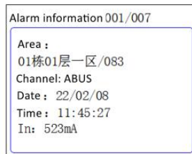
Residual current alarm
