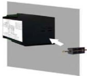
Step 3: Tighten the screws of the fixture clockwise with a screwdriver until the controller is firmly installed.
