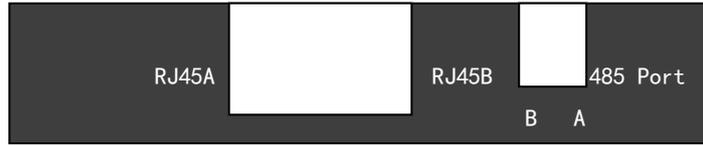
The output terminal has two RJ45 network interfaces. Take over any one to the RJ45 port of intelligent capacitor; 485 interface to a computer.
